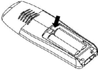
Fit the battery compartment cover, sliding it until it clicks firmly into Position.
